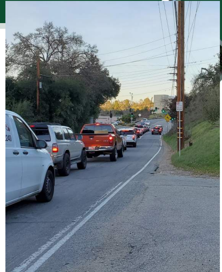
Traffic demand exceeds available turn lane storage - Mulholland Hwy at Old Topanga Canyon Rd (East)
