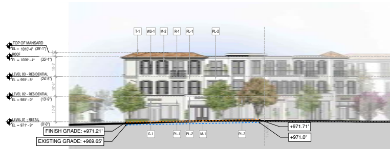
5 Building B-2 South-West Elevation SCALE: 1/16"=1'-0"
