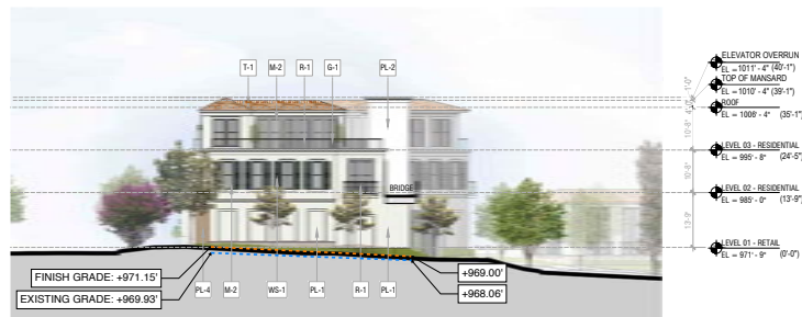
2 Building B-2 East Elevation SCALE: 1/16"=1'-0"
