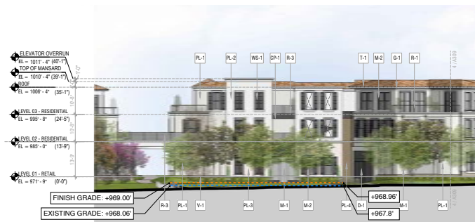
3 Building B-2 North Elevation SCALE: 1/16"=1'-0"
